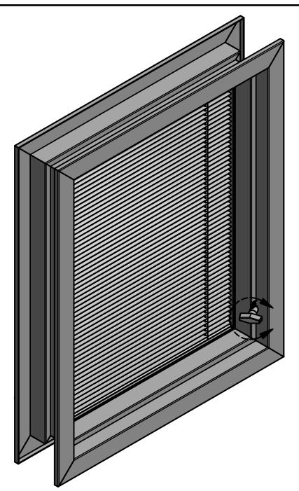
ADA COMPLIANT TILT CONTROL KNOB ASSEMBLY (BY KYLER INDUSTRIES) -LOCATION TO BE ANY WHERE ON VERTICAL SIDE OF FRAME - AVAILABLE IN SINGLE OR DUAL OPERATOR
