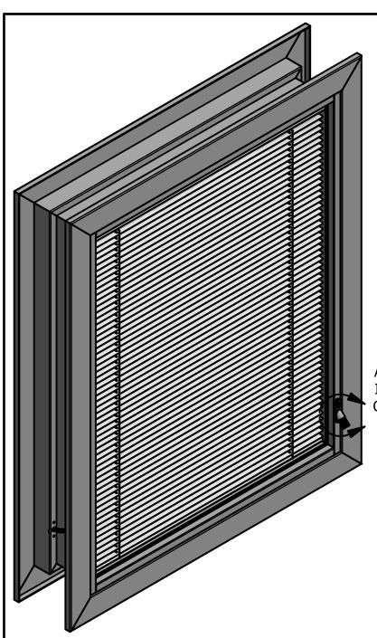
ANGLED DOWN TILT CONTROL KNOB ASSEMBLY (NOT ADA COMPLIANT) (BY KYLER INDUSTRIES) - LOCATION TO BE ANY WHERE ON VERTICAL SIDE OF FRAME - AVAILABLE IN SINGLE OR DUAL OPERATOR
