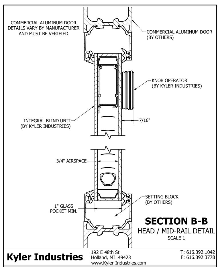
SL20A Integral Blind; Commercial Aluminum Door; Knob Operator; Tilt Only
