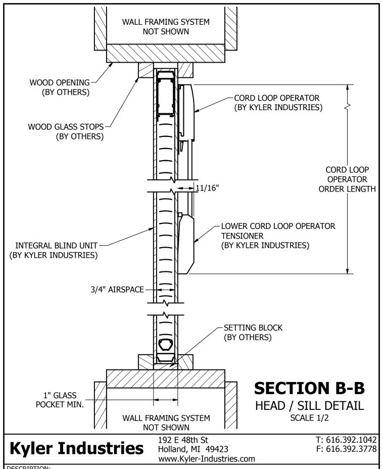
SL20 Integral Blind; Wood Opening; Cord Loop Operater; Tilt Only (SL20A) or Lift/Tilt (SL20C)
